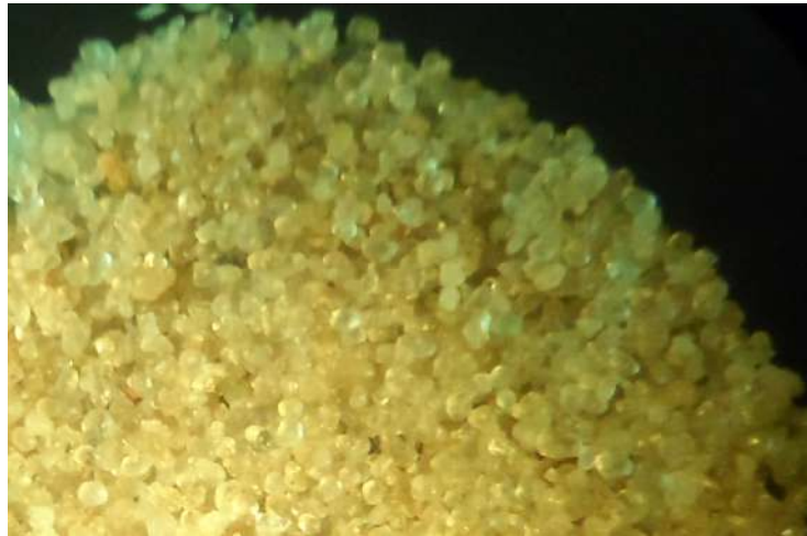
Figure 5 – Photo of the surface of foundry core through an optical microscope (increase 14 times)
