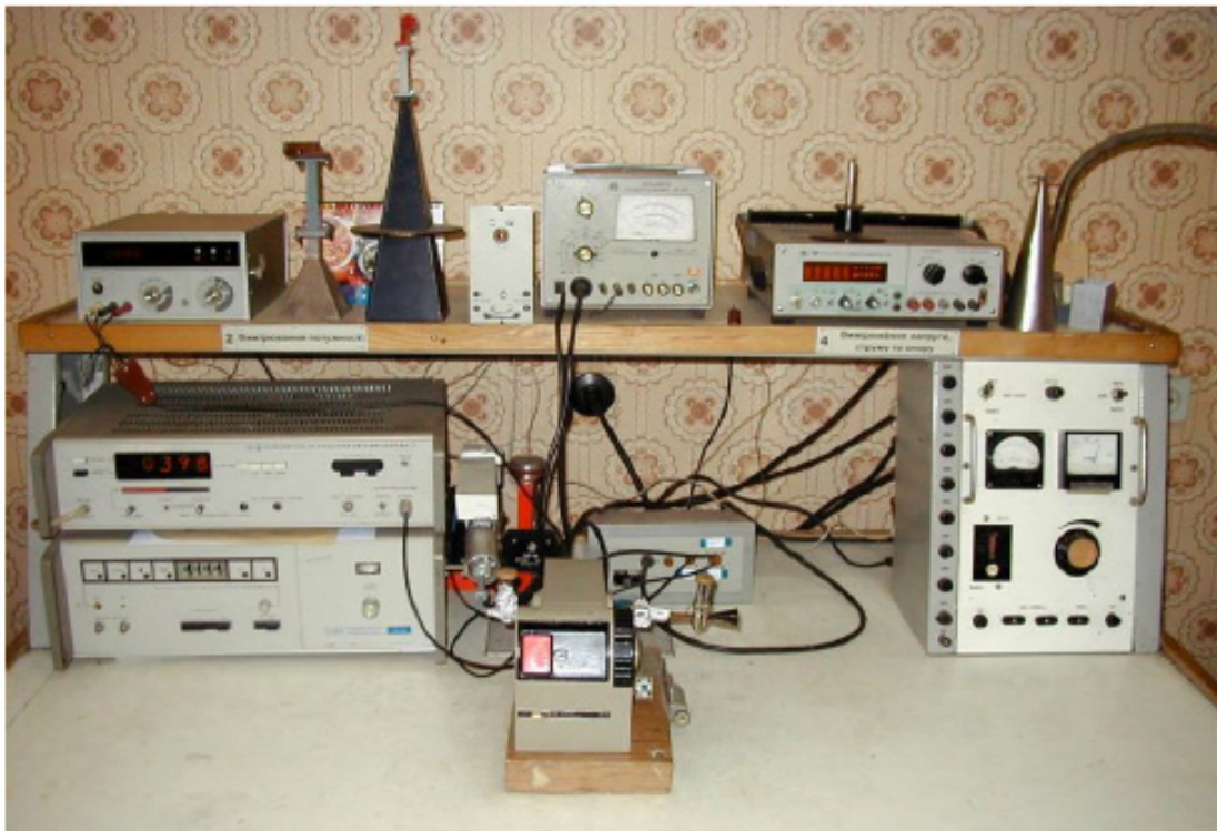
Figure 1.5 – Appearance of the radiometric unit on frequency bands 37...53 GHz
