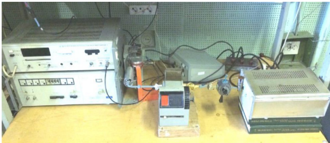
Figure 3.24 – A workstation for checking a high-sensitivity radiometric system for 37...53 GHz frequency range using a standard noise oscillator G_n (right)
