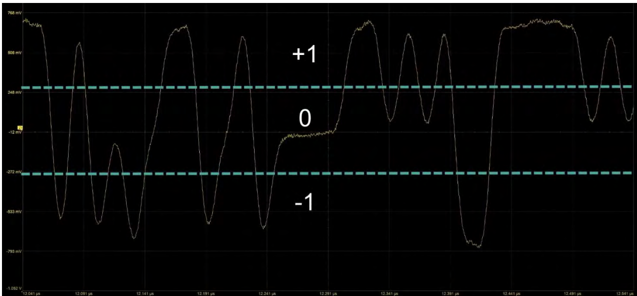
Figure 2 Example of signal conversion in PAM3
