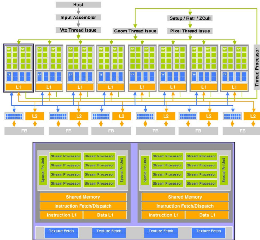
Figure 2.3 – GPU Streaming Multiprocessor Structure
