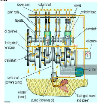
There is an oil pressure sensor near the oil pump that monitors pressure and sends this information to a warning light or a gauge on the dashboard. When you turn the ignition key on, but before you start the car, the oil light should light, indicating that there is no oil pressure yet, but also letting you know that the warning system is working. As soon as you start cranking the engine to start it, the light should go out indicating that there is oil pressure.
