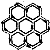
Fig. 7. Circular Ampere current in a magnetized bar (viewed from the pole).
