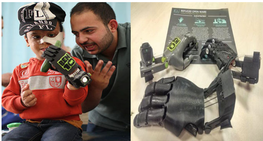
Fig. 5.8 ROW 3D printed prosthetic hand (3D Printing and Prosthetics, 2017; Refugee Open War, 2017)
