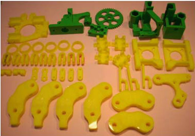
Fig. 2.9 RepRap self-replicated plastic components (Romero et al., 2014)
