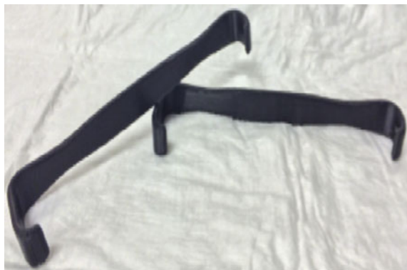
Fig. 4.2 3D-printed polylactic acid Army-Navy surgical retractor (Rankin et al., 2014)
