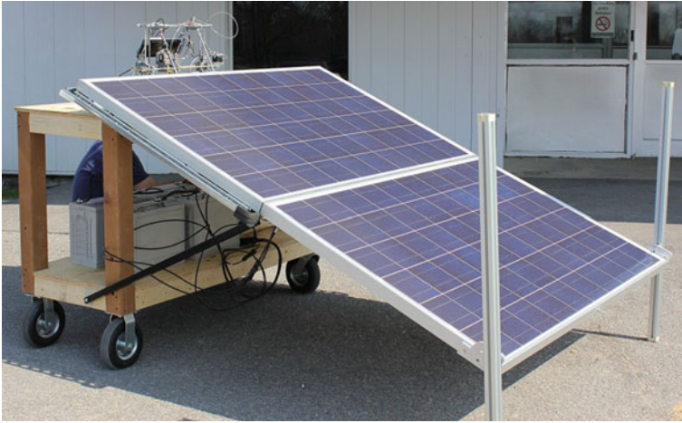
Fig. 5.3 Community-scale solar-powered open-source RepRap 3D printer system for off-grid communities (King & Babasola, 2014)
