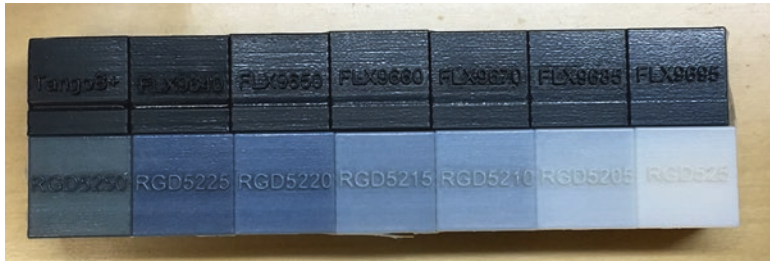
Fig. 2.8 High-end material jetting printers allow printing models using mixtures of two to four base resins loaded into the machine. Here, 14 cubes were printed in a machine with two material heads, one loaded with a flexible black-colored material (cube in top left corner ) was printed with that material at 100%) and the other loaded
