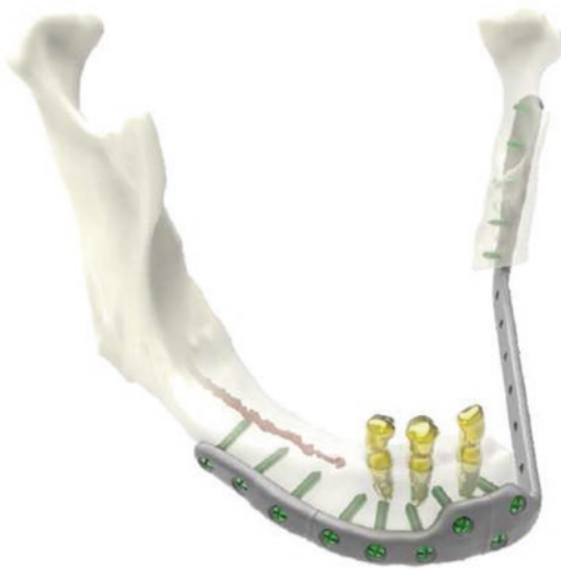
Fig. 9.13 3D Printed mandibular reconstruction plate (gray) following a resection of the left mandible. Precise screw locations and contour can be achieved by the combination of digital design and digital output. Courtesy KLS Martin, Jacksonville, Florida, USA
