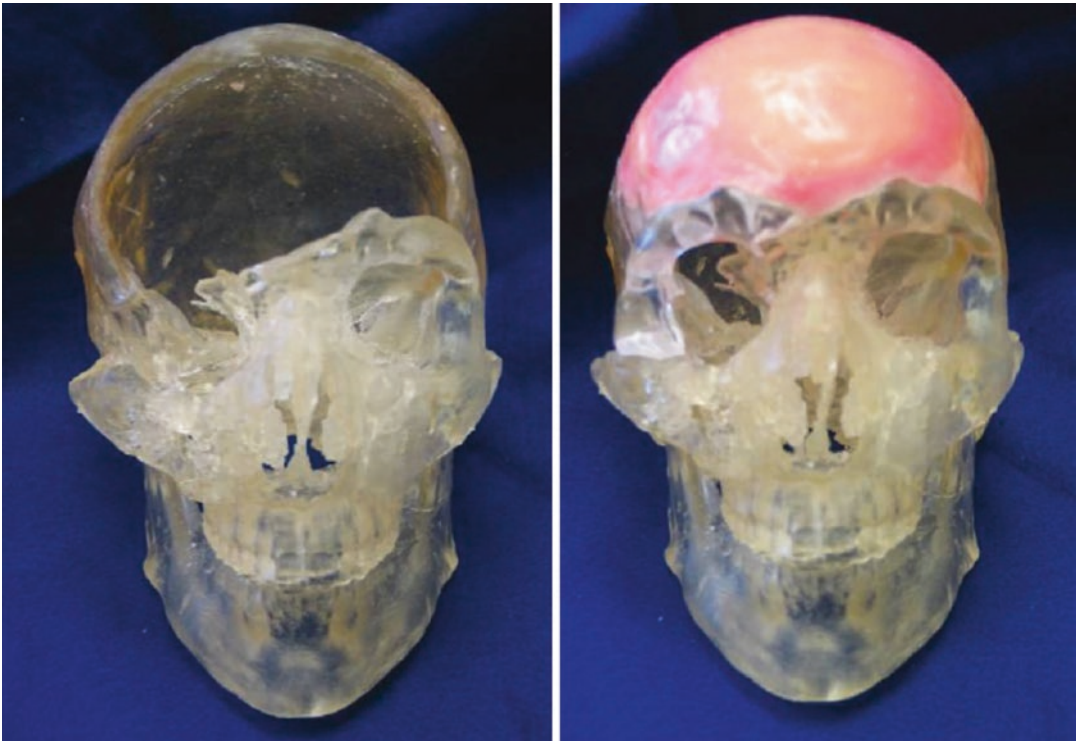
Fig. 5.2 The left photo is the SLA skull with a frontal bone and lateral orbit defect. The right is the waxed implant for mold fabrication
