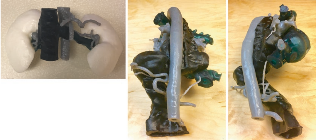
Fig. 2.6 Example of model of a bilateral renal aneurysm printed with vat photopolymerization ( left-hand panel ) with arteries printed in gray , veins in black , and kidneys in white . Each component was printed separately using the different-colored resins and later meticulously assembled together. This is not always readily (or at all) possible as
