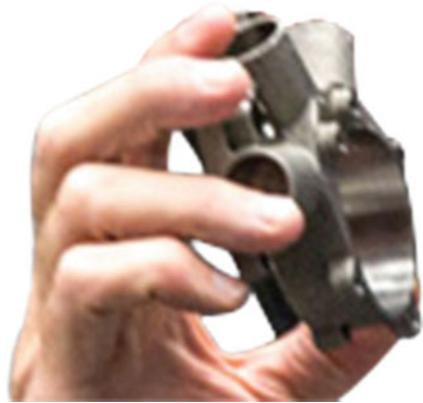
material waste. At present, the company is metal 3D printing technology to develop 3D printed satellite parts (as shown in Fig. 8) and plans to increase the process to manufacture complex parts in the future [9].
