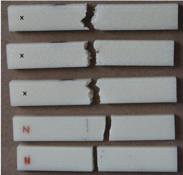
**Fig. 12** Failure pattern of the fractured test samples
