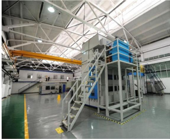
Northwest Polytechnic University (NPU) has developed the production of large-scale laser cladding cell. The laser-cladding cell can build a part size of  $5 \times 2.5 \times 0.6$  m; accuracy of deposition speed is  $\pm 1$  mm and an inert atmosphere of 50 ppm (shown in Fig. 16).
