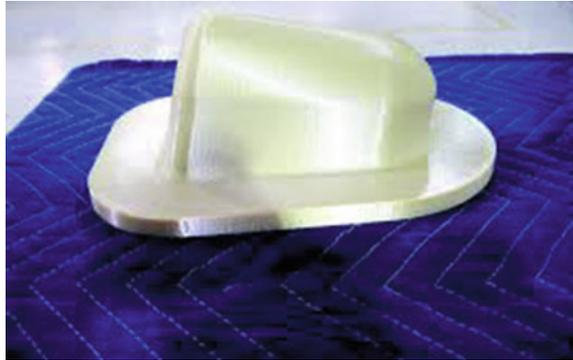
**Fig. 7** FDM-layup tool produced the aircraft camera fairings
