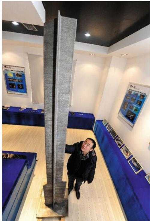
During 2013, Northwest Polytechnic University (NPU) Laser Cladding Cell has developed central wing spar for 'Comac C919' passenger-plane and it is predicted to enter the commercial service in 2016. The length of this central wing spar is 5 m and having mechanical properties equal to forging parts as claimed by the NPU University (shown in Fig. 17).
