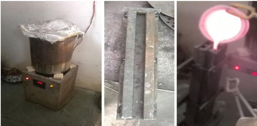
**Fig. 2** Electric muffle furnace, Mould, and Casting process
