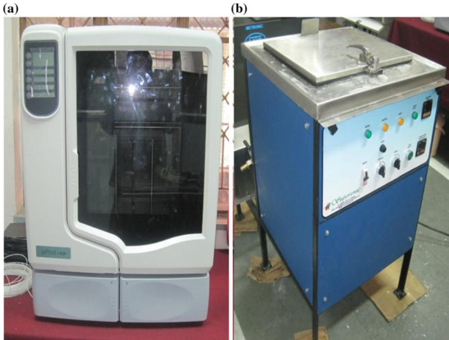
**Fig. 7** **a** RP FDM machine (uPrint, Stratasys), **b** agitation tank (Biosonic)
