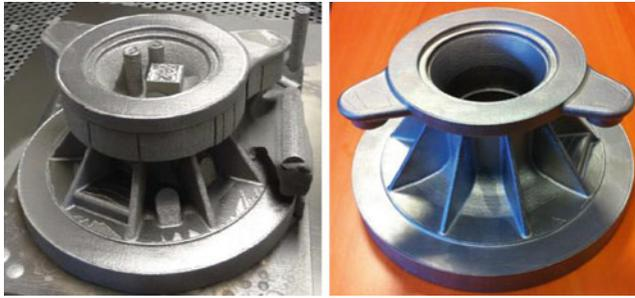
**Fig. 4** Turbo-pump housing made in TA6V by EBM process
