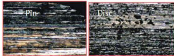
The track surface for test no 6 reveals a lot of binder particles visible as black color spherical shapes. These particles were used as binders in the metal powders during manufacturing of the test specimens. These particles come from the wearing of the pin specimen. The particles are present in spite of the track being continuously cleaned. This results in the pin specimen sliding against particles of its similar kind, hence there is reduction in wear.
