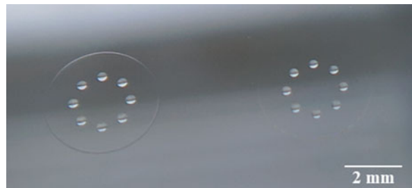
Fig. 2 Photograph of ductile-cut microlens arrays on a silicon wafer
