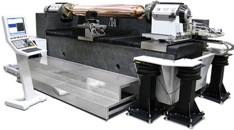
Fig. 10 A roller mold installed on an ultraprecision CNC horizontal drum lathe (Zhang et al. 2014)
