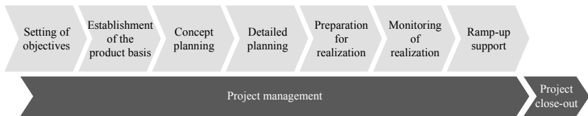
Figure 16: Phase model of the factory planning process (VDI 5200, Part 1, p. 9)
