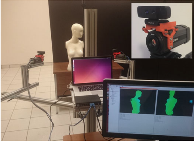
Fig. 6 Photograph of the 4D thermography system with two camera units mounted on rotating arms around a subject, each camera unit (inset photograph) consists of a FLIR A320 thermal imaging camera and a Creative Senz3D depth sensor
