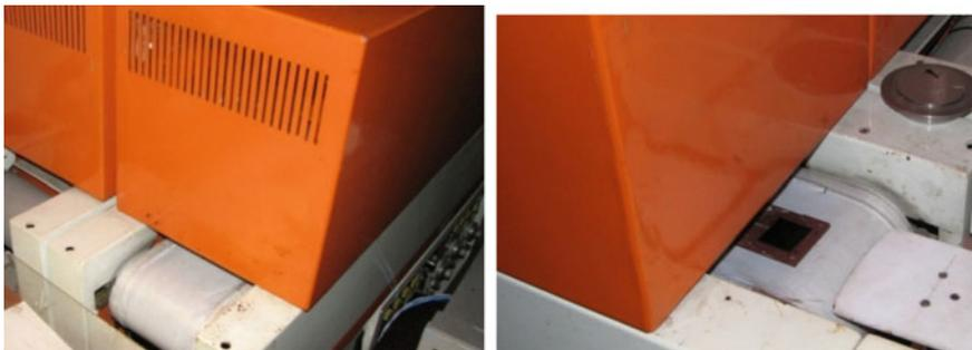
**Fig. 4.17** “LADA” desiccation system: *left-inlet part; right-outlet part (with wafer coming out)*
