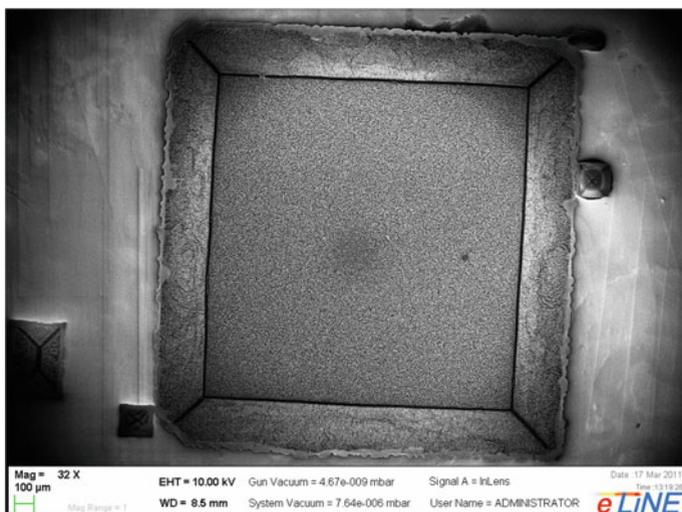
**Fig. 4.26** Membrane with 0.4 mm side lengths
