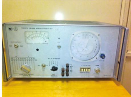
In the hot imprint process experiment frequency generator Г3-56/1 was used (Fig. 5.48).
