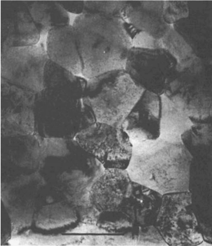
Fig. 14.26 TEM of a sample strained to 97% at 1327 °C. I_0 = 1.2 \times 10^{-4} /s. Scale bar = 0.5 \mu\text{m} . Duclos et al. [8]. With kind permission of Elsevier
