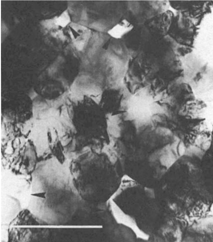
Fig. 14.29 TEM of a sample strained to 82% at 1297 °C. Cavities are indicated by arrows . \dot{\epsilon}_0 = 1.2 \times 10^{-4} \text{ s}^{-1} . Scale bar = 1 \mu\text{m} . Duclos et al. [8]. With kind permission of Elsevier
