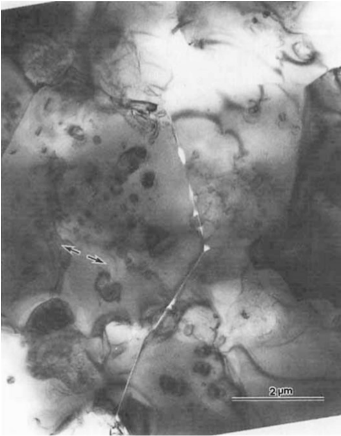
Fig. 6.12 Transmission electron micrograph of a trace of intergranular crack propagation. The sample was tested at 1220 °C and 100 MPa in tension. Note the transgranular fractured nanoparticle. The stress direction is indicated by an arrow . Ohji et al. [11]. With kind permission of John Wiley and Sons
