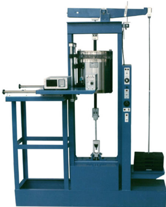
Fig. 5.1 Special Series 2330 Lever Arm Creep Tester designed for tensile testing of ceramic specimens. Features include a high-temperature furnace and integrated slide table for use with non-contacting laser extensometer. With kind permission of R. Antolik of Applied Test Systems Inc.
