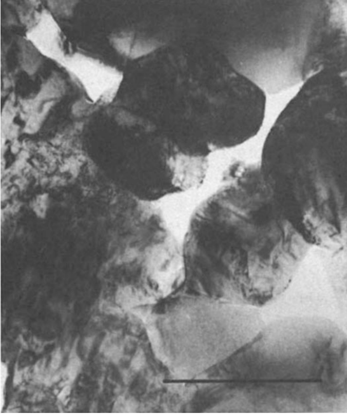
Fig. 14.28 TEM showing cavities in a sample strained to 40% at 1223 °C. \dot{\epsilon}_0 = 2.4 \times 10^{-5} \text{ s}^{-1} . Scale bar = 0.5 \mu\text{m} . Duclos et al. [8]. With kind permission of Elsevier
