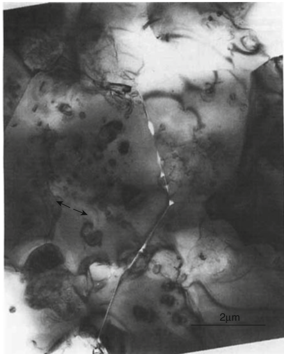
Fig. 12.72 Transmission electron micrograph of a trace of intergranular crack propagation. The sample was tested at 1200 °C and 100 MPa in tension. Note the transgranular-fractured nanoparticle. The stress direction is indicated by an arrow. Ohji et al. [19]. With kind permission of John Wiley and Sons
