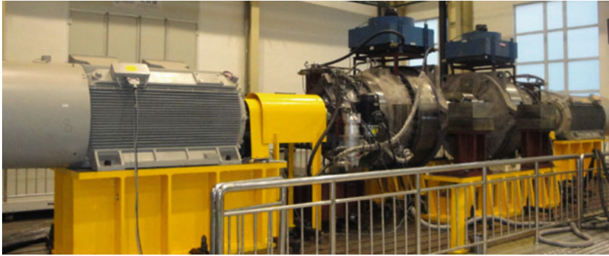
Fig. 6.1 Bench test of a wind turbine gearbox
