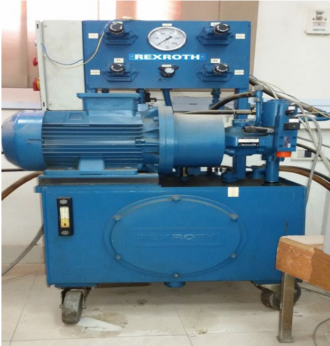
Fig. 14 Hydraulic power unit
