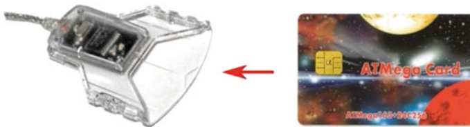
Fig. 4.2 Connect the card reader to your computer and insert the SmartCard into the reader
