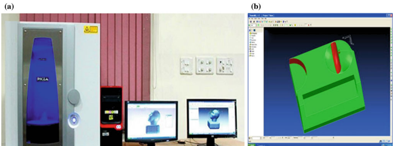
Fig. 5.5 a PICZA 3-D Laser scanner LPX-600 acquiring some images. b Delcam module performing auto-coding on scanned data of an engineering part
