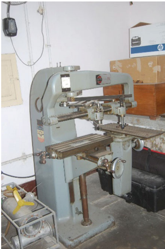
Fig. 7.3 A panto mill-cum-engraving machine. [Make: panto mill gorton, size of work table: 8" X 18", cross travel = 8" & vertical travel = 10", pantograph ratio = 1:2 & 1:16]
