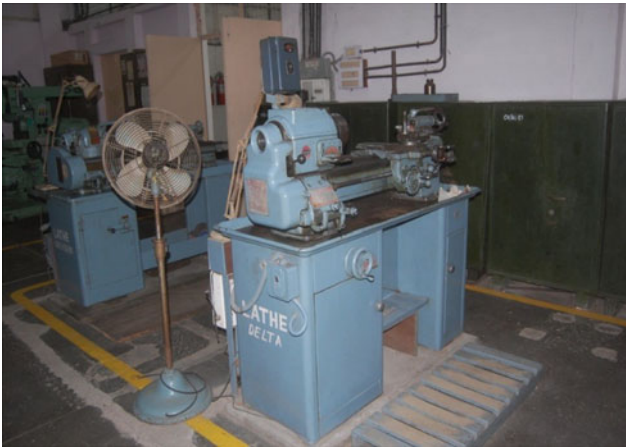
Fig. 7.2 A multipurpose delta lathe machine. [Make: rockwell, swing over cross slide: 150 mm, swing over saddle: 245 mm, distance between centre: 800 mm, spindle speed = 45–1550 rev/min]
