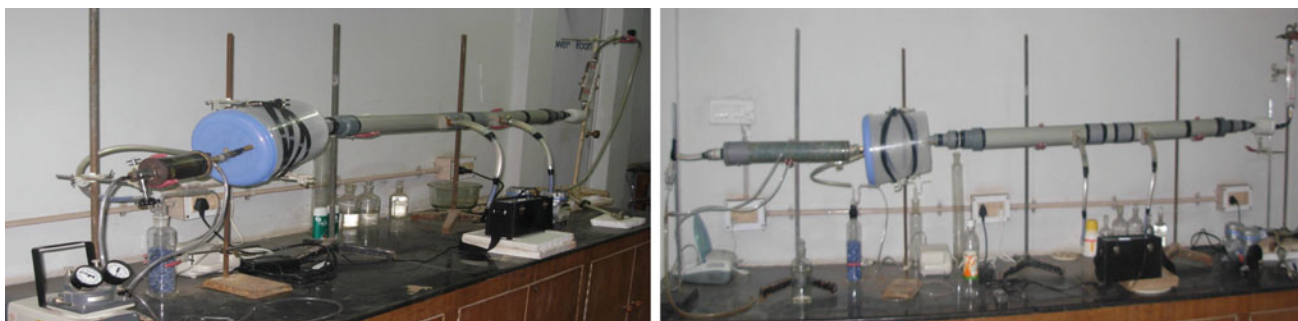
Fig. 3.2 Dry and wet aerosol generation system and impactor testing rig
