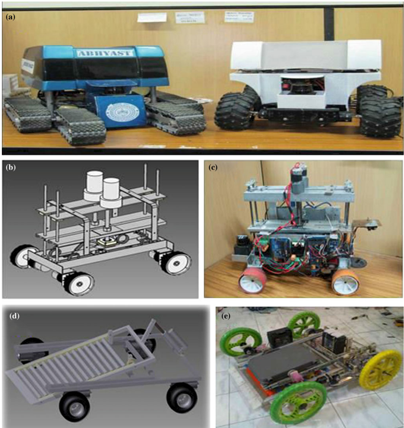
Fig. 5.11 a Phase 1 and 2: rough terrain vehicle with obstacle avoidance. b CAD model of Phase 3 (ANS). c Phase 3: ANS with jumping capability. d CAD model development for ground vehicle.
