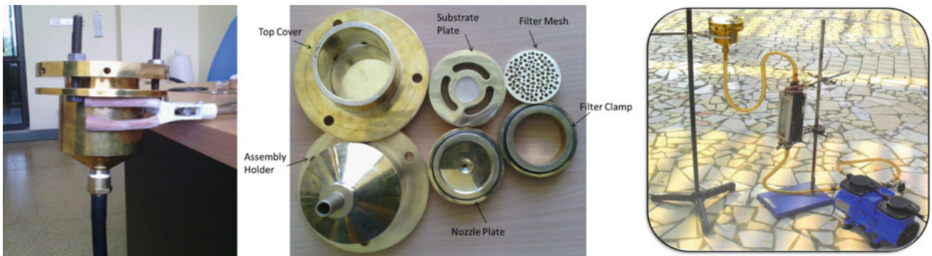
Fig. 3.5 Developed PM 1.0 sampler with its internal components and its field setup
