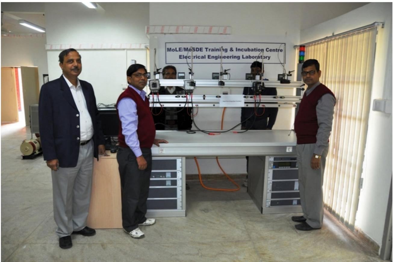
Fig. 1.2 Energy meter test bench in old SAC
