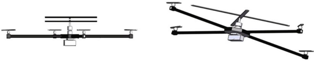
**Fig. 1.4** A compound multicopter. The middle coaxial propellers with a slow dynamic response provides the main lift, while the surrounding quadcopter can change the propeller angular speeds rapidly to improve the dynamic response of attitude
