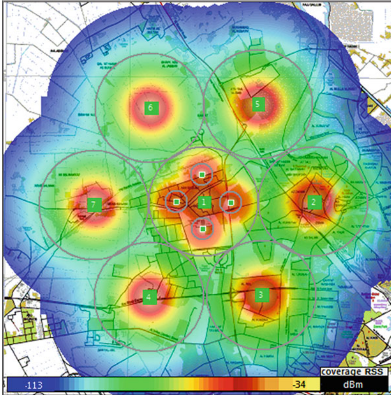
Fig. 4.4 Gradient color of coverage area distribution for four RN deployed located at 1250 m from BS with 10 W transmission power as Case 1 in Table 4.1
