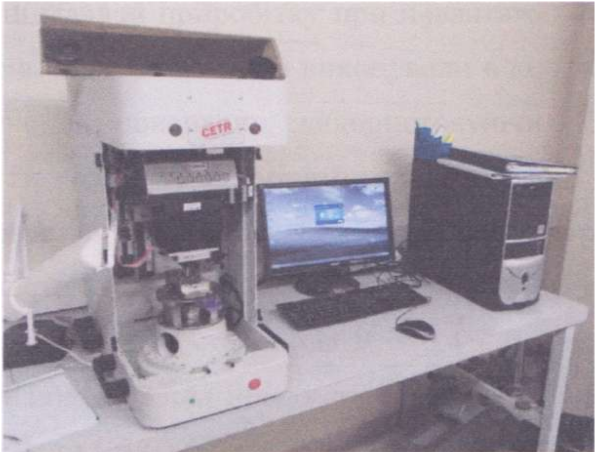
Figure 4.8 – Bruker UMT Multi-Specimen Test System tribotester
